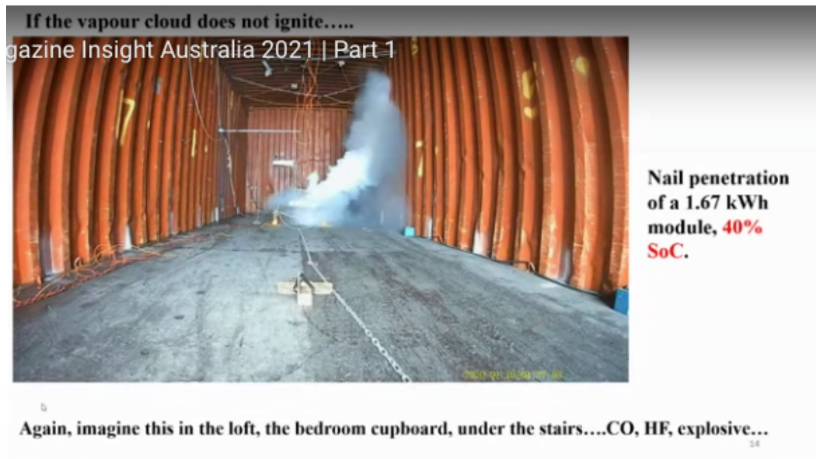
Figure 5 (c): The white vapour cloud follows a fraction of a second later. The light-scattering material creating the opaque white material is likely to be the organic solvents from the cell.
