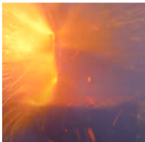
Figure 1: (a) A charged 2.6 Ah cell being deliberately overheated. (b) at the point of rupture (c) the cell takes off as a rocket (d) seconds later the discharge is complete, and the cell is red hot. 5:56 mins to 6:24 mins.
