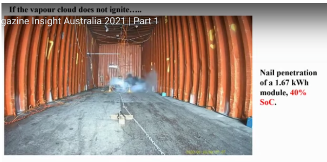
Figure 5 (b). Initial failure of a 1.67 kWh module in a low State of Charge (SoC) (40%). The black cloud (said by Christensen to be “cathode material”) emerges in the first fraction of a second.
