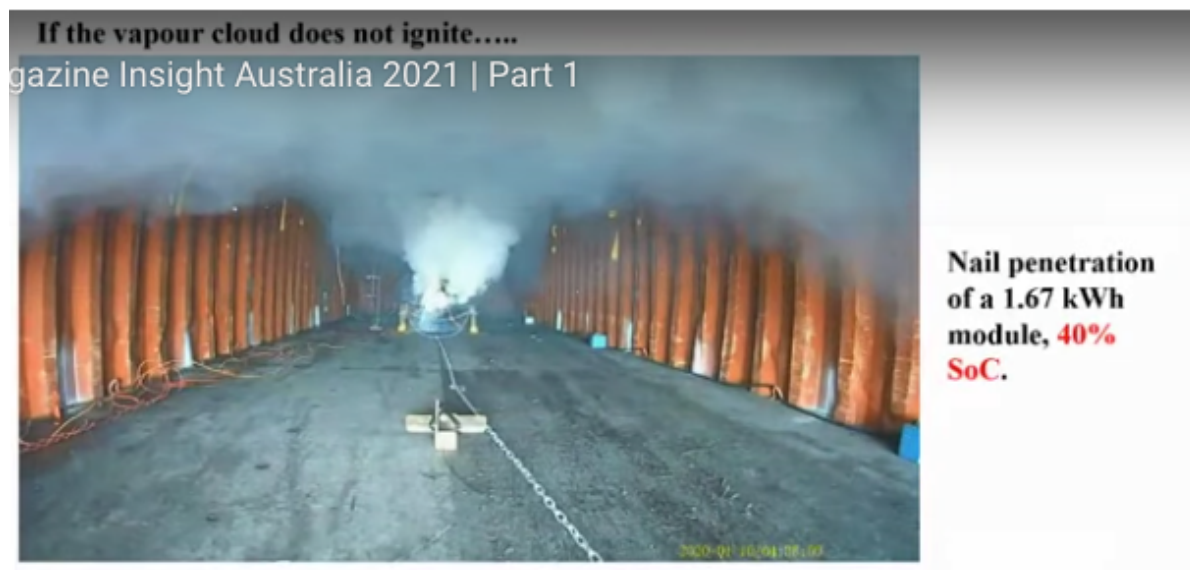
Figure 5 (d). The vapour cloud eventually fills the container, without ignition, during the test.
