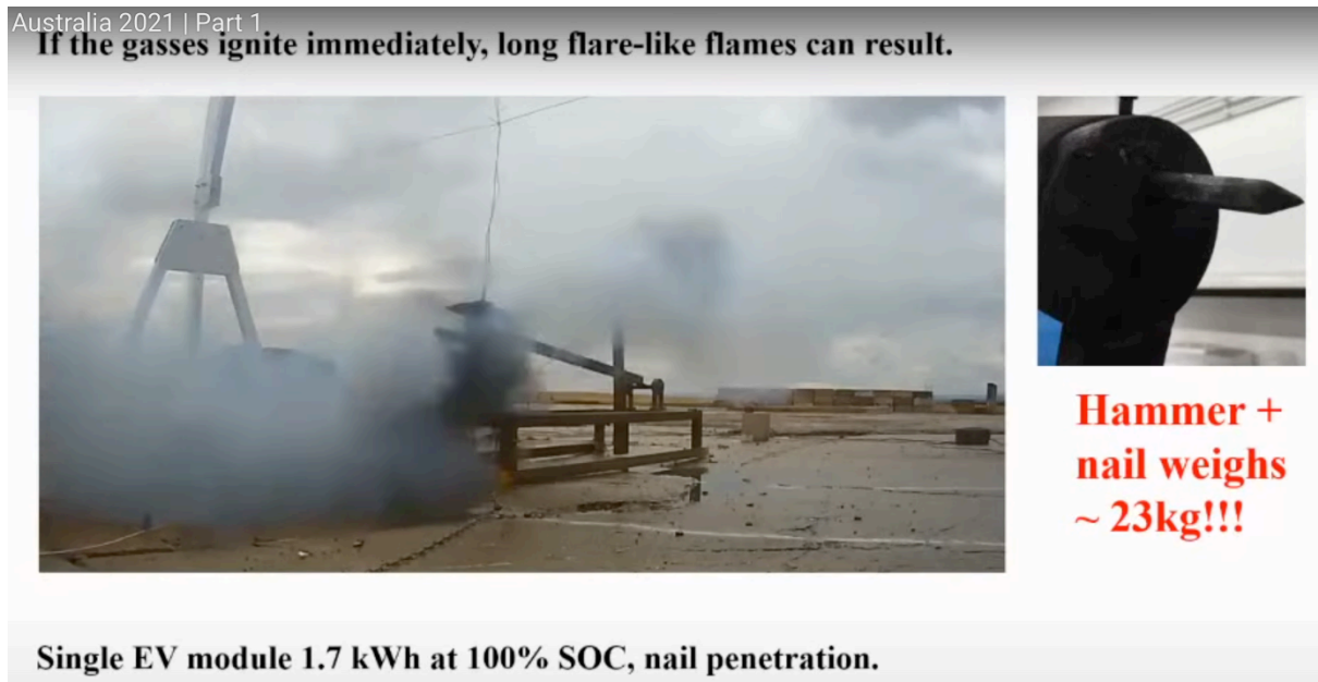
Figure 3(d). A fraction of a second later, a black cloud of what is said by Prof Christensen to be “cathode material” emerges.
