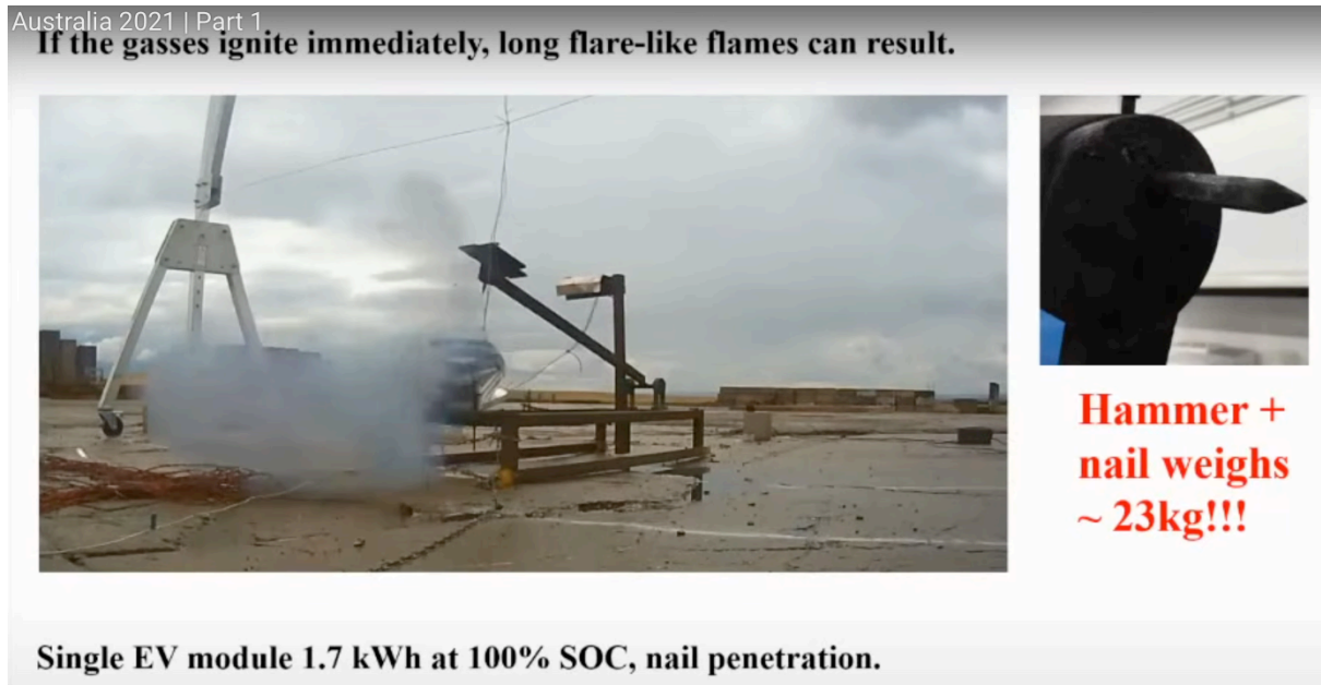
Figure 3 (c). The hammer of 23 kg weight is thrown back into the air as the cells in the EV battery module disrupt explosively:
